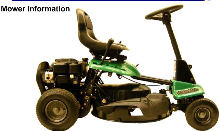
The LRV has a 26 inch single blade mower with vents.
