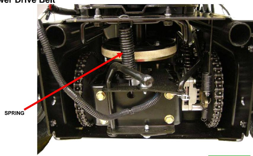
Remove the spring that pulls the rubber wheel against the steel disc.
