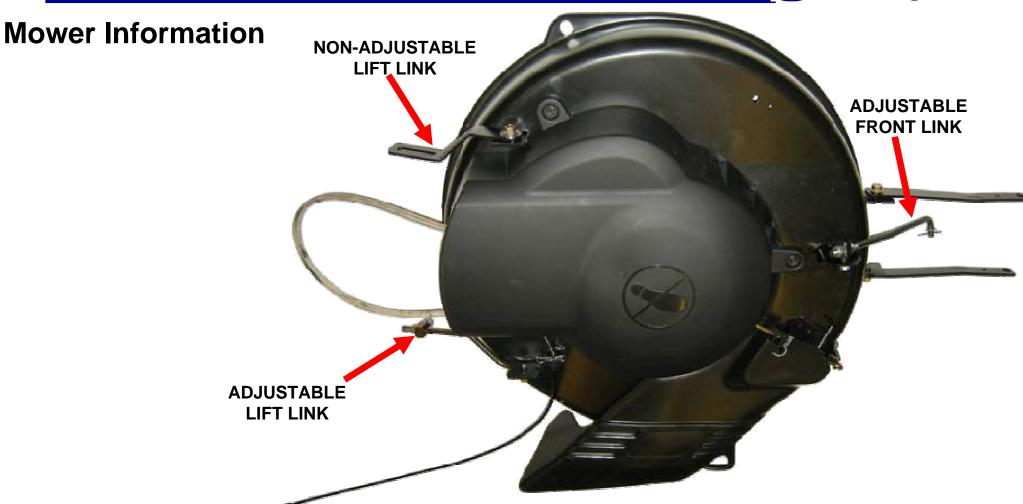
The suspension is similar to other Husqvarna tractor mower decks with an adjustable front link, a non-adjustable lift link, and an adjustable lift link.
