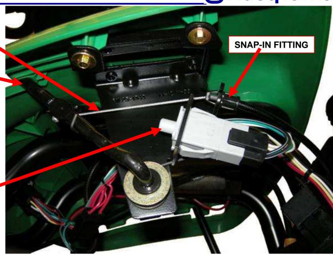
The mower engagement cable is shown where it attaches to the mower engagement lever. **RETURN TO**
