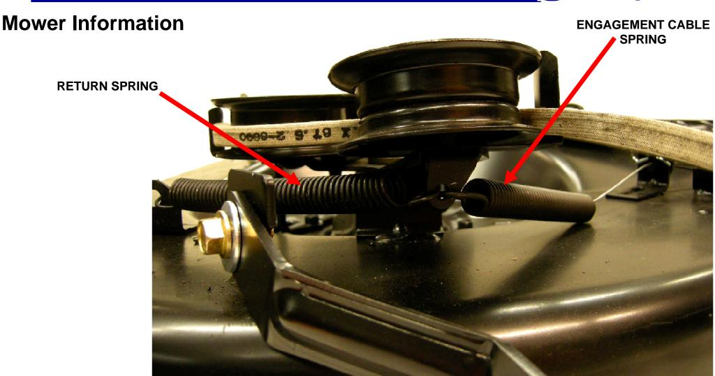
This picture shows the attachment points for the return spring and the spring on the end of the engagement cable.
