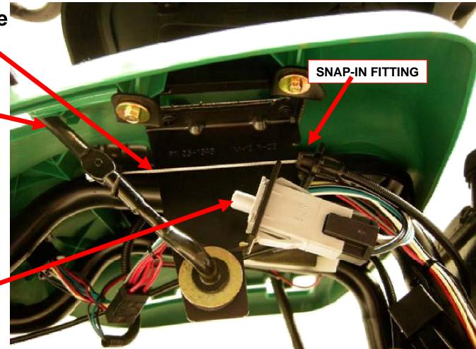
The mower engagement cable is shown where it attaches to the mower engagement lever. **RETURN TO**
