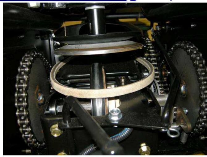
Remove the belt from the pulley.
