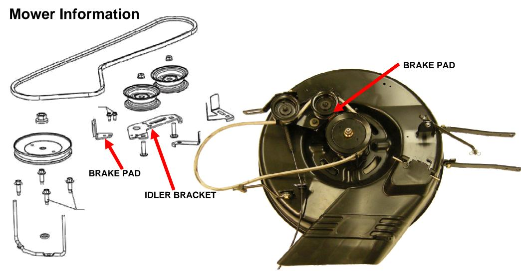
The mower deck is operation is straightforward. Note that the brake pad is replaceable and attached to the idler bracket.
