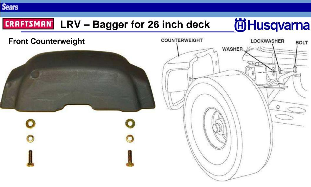
The front counterweight is installed to the front axle with a screw, lockwasher, and washer on each side.
