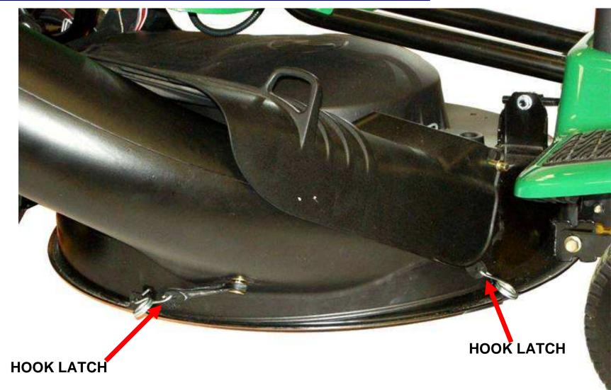
• Use the hook latches to secure the lower chute to the mower deck.
