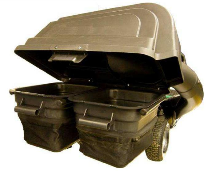
• The grass containers install into the bagger cover.
