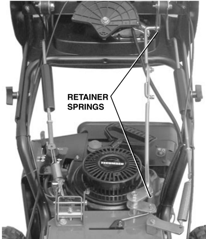
3. To replace Speed Control Assembly, remove both 5/16" screws securing the Drive Speed Control Lever to the Console Panel. Hydro models have four of these screws (see the illustration on Page 33, Key #2).
