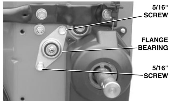
6. Remove the Flange Bearing and Hex Shaft (as an assembly) from left side of snowthrower.
