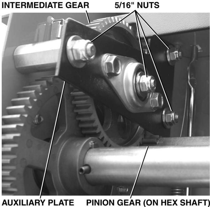
6. Remove Bolt from old Intermediate Gear and install on new Gear.
