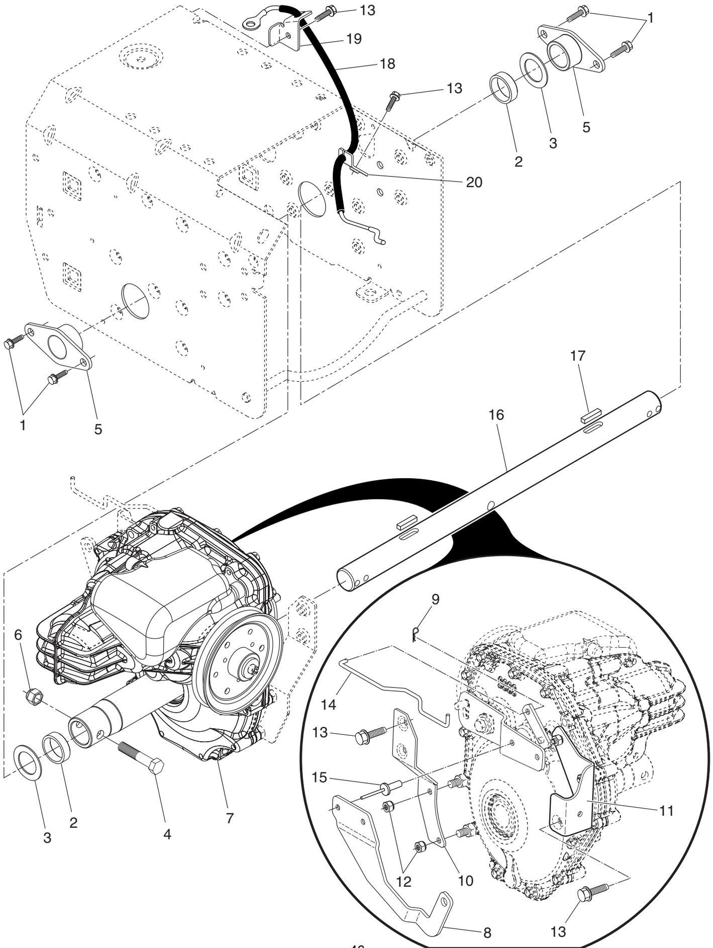
**NOTE:** The hydro transmission is a sealed, self-contained unit. It does not require additional fluid or lubrication. There is no way to check the fluid level in the transmission. If a serious leak develops and a significant amount of fluid is lost, the hydro transmission should be replaced.
