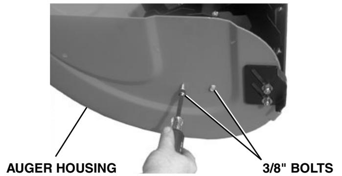
6. Remove the Augers, Impeller, Gearbox and Auger Bearings from the Auger Housing as an assembly.
