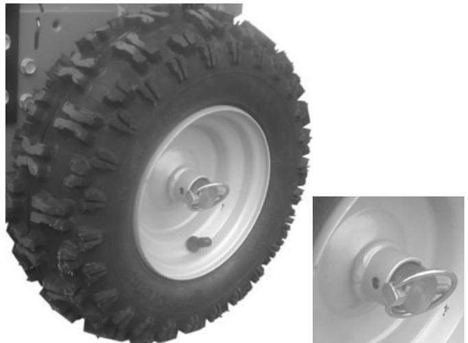
**NOTE:** To push the snowthrower easily (“free-wheeling” mode), install the Klik Pin in the outer axle hole, with the wheel hub to the inside.
