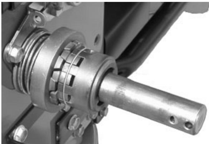
5. Reinstall Hardened Thrust Washer (Page 36, Key 28), Axle Lobe (Key 26), Wheel Lobe (Key 23), and Retaining Ring (Key 33).
