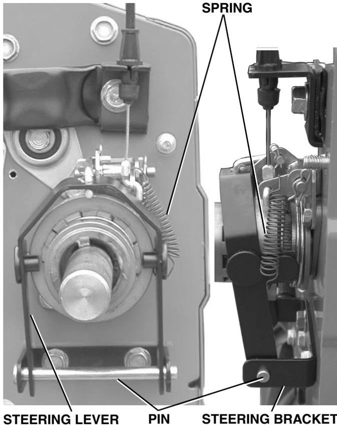
3. Remove Retainer Spring securing Steering Link to Bellcrank, then remove Steering Link from Bellcrank.
