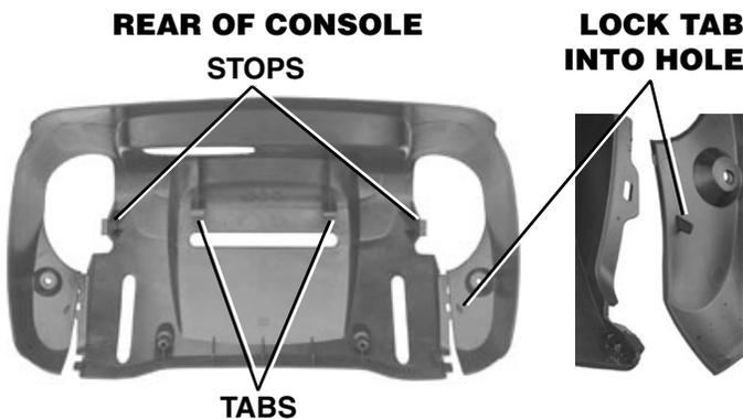
4. Reverse the above steps to reassemble. Be carefull not to overtighten the screws.
