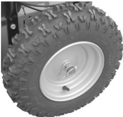
**NOTE:** Klik Pin must be in this position only for the Power Steering to work. The hole in the wheel hub is **NEVER** used on Power Steering models.
