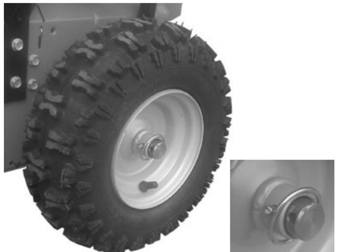
**NOTE:** For the wheel to drive, the Klik Pin must be installed through both the wheel hub and the inner axle hole.
