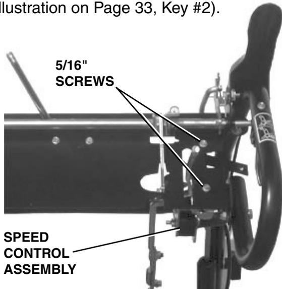
6. Reverse the above steps to reassemble. Be sure to readjust linkage (see Section 6.24).
