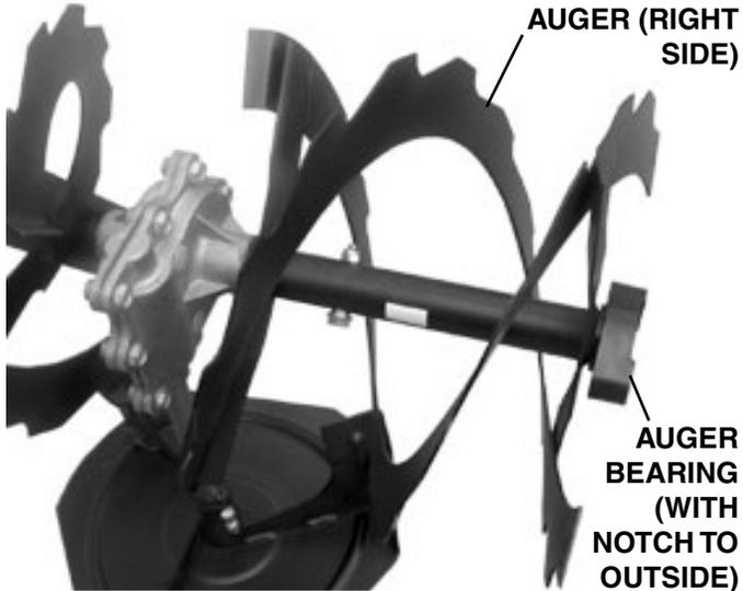
**NOTE:** Be sure the LH Auger is on the LH side. Stamped into the end of each auger “flight” is an “L” or a “R” for Left or Right side. The stamped number is the auger width in inches.
