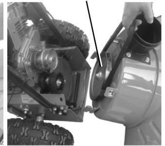
8. Ensure that Idler Spring is in place before re-attaching Auger Housing to snowthrower. Put tape over the spring hook (on outside of housing) to keep spring in proper position.
