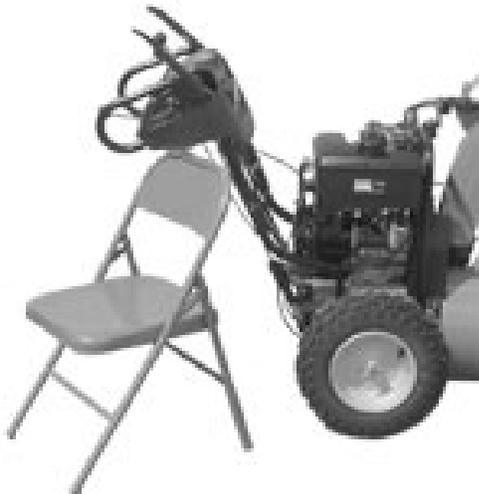
6. Remove Auger Belt from Auger Pulley.
