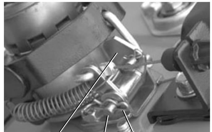
9. Remove 5/16" screws securing Turn Trigger to Handle. Remove cable from Turn Trigger.
