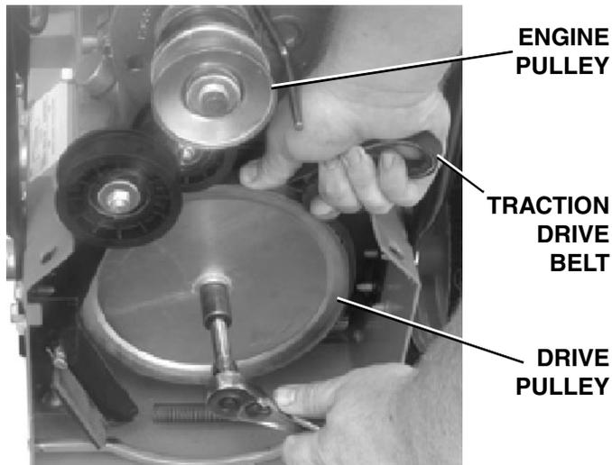
4. Put anti-seize compound on the bolt before installing new Drive Pulley. Reinstall bolt and washer. Torque to 15-20 ft. lbs.
