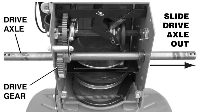
5. Inspect parts for wear, replace as required.
