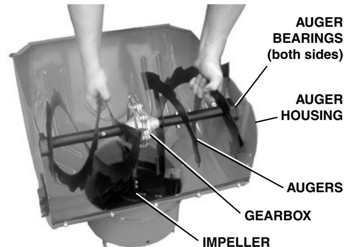
7. To replace an Auger, remove the Shear Bolt on the appropriate side and slide Auger off of the Auger shaft.
