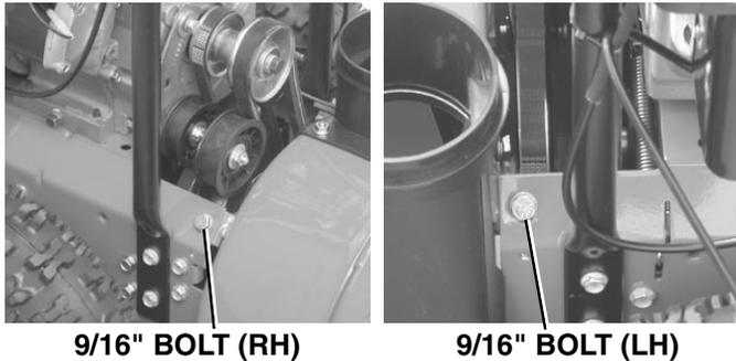
5. Separate Auger Housing from snowthrower. Use a chair or saw horse to support handle.
