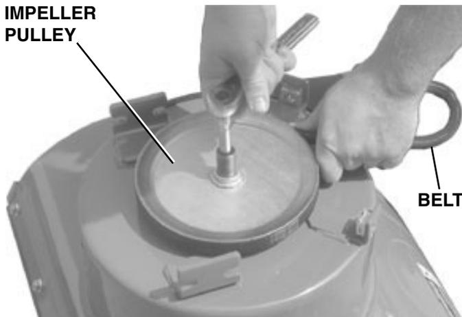
3. Remove the Impeller Pulley from the shaft. A gear puller may be required. If so, it will help to put a socket between the screw of the gear puller and the shaft.
