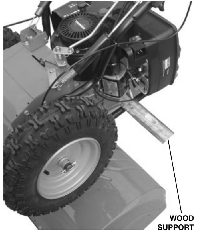
10. Use a 1/2" socket with 15" extension to remove Engine mounting bolts (Page 35, Key 16).
