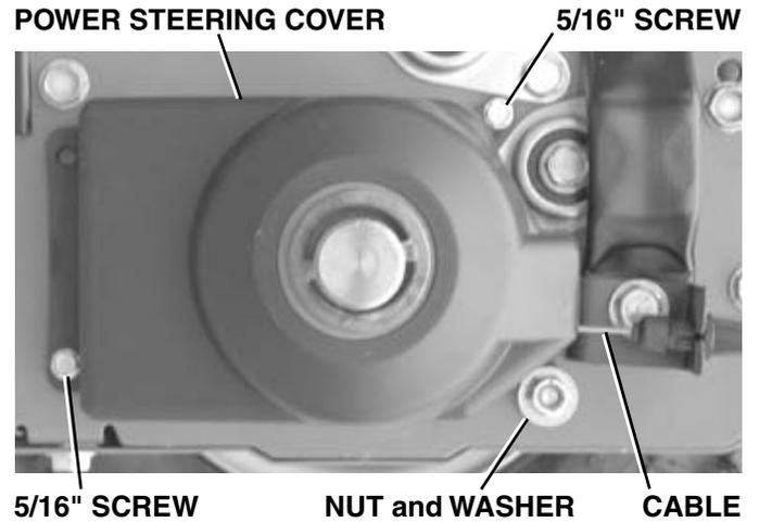
4. Note the routing of the Power Steering Control Cable and the locations of plastic ties securing it. Cut all plastic ties, then remove cable.
