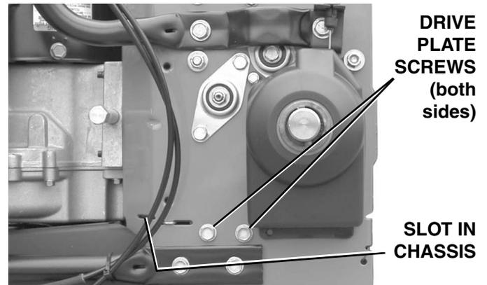
5. Remove Drive Belt from pulleys. You can now remove the Drive Plate.
