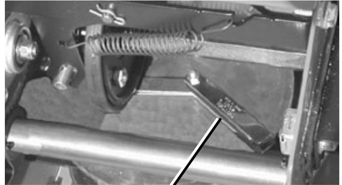
2. If the rubber ring on the traction disc is missing chunks, has deep cracks, or is worn to the point where the rubber ring clamp plates are 1/16" or less from the drive plate (in engaged position), the rubber ring must be replaced.
