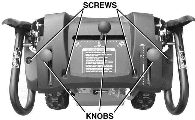
3. Carefully separate lock tab at each side and remove Console Panel from snowthrower. (Check picture below for position of tabs and stops on the back side of Console Panel).
