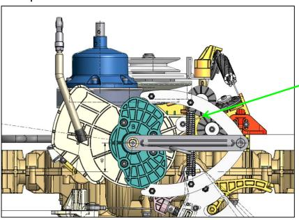
Cable attachment must be aligned between the both roller (see line on the drawing below)
