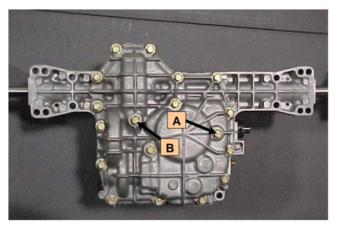
**Location A = Drains oil from Hydrostatic compartment.**
