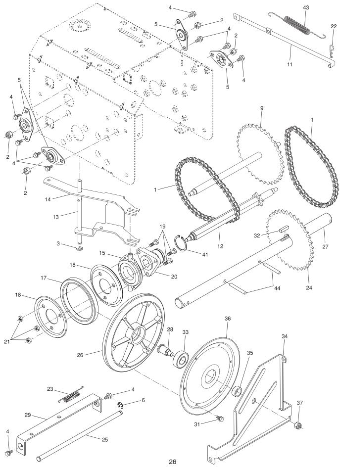
**REPAIR PARTS** SNOW THROWER - - MODEL NO. **PR5524ES** (96192001600) DRIVE
