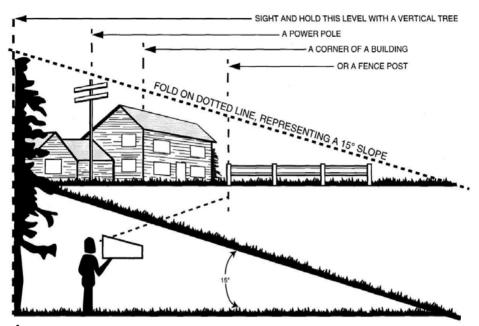
**WARNING:** Do not mow a slope that has an angle of greater than 15° (a rise of approximately 2 1/2 feet [.75 m] every 10 feet [3 m]). Mow across the face of a slope, and never up and down.
