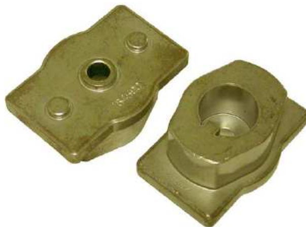
Part # 184598 Shaft Depth 1.0 inch Part # 184590 Shaft Depth 7 / 8 inch 25 mm Crankshaft Torque GR8 bolt at 35-40 Ft. Lbs
