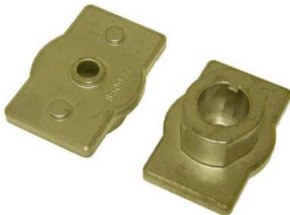
Part # 850977 Shaft Depth 1.0 inch Part # 851514 Shaft Depth 7 / 8 inch 7/8 inch Crankshaft Torque GR8 bolt at 35-40 Ft. Lbs
