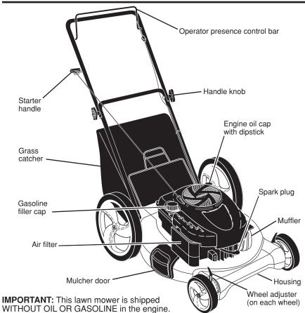
NOTE: Gasoline containing up to 10% ethanol (E10) is acceptable for use in this machine. The use of any gasoline exceeding 10% ethanol (E10) will void the product warranty.
