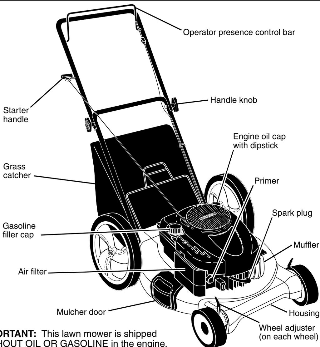
**IMPORTANT:** This lawn mower is shipped WITHOUT OIL OR GASOLINE in the engine.
