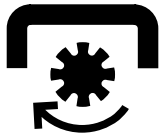
ATTACHMENT CLUTCH ENGAGED
