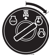
ENGINE "ON" POSITION (NORMAL OPERATING)
