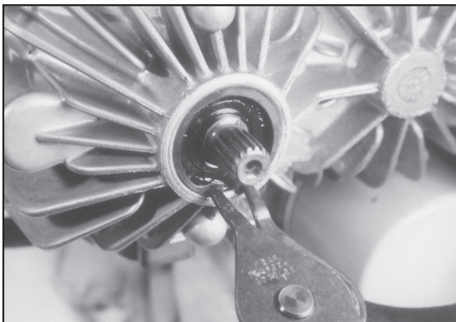
Retaining Ring Installation
