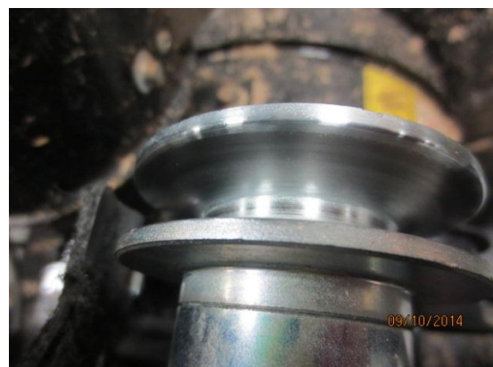
After – shiny and smooth v-groove surface
